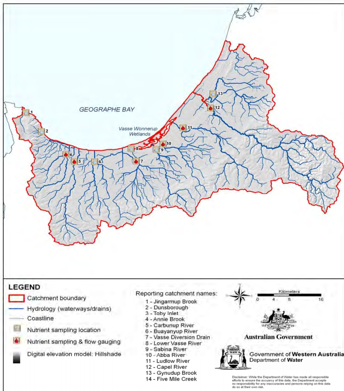
Figure 7: The location of water quality monitoring points in the Geographe catchment sampled for the Coastal Catchments Initiative project.
