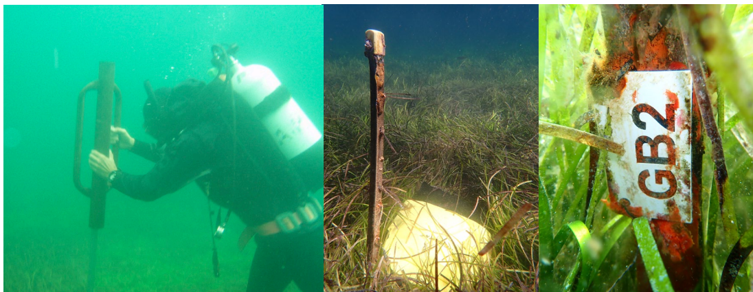
Figure 2: Left: Banging in permanent marker with pole driver. Middle: Star picket with cap indicating centre of 50 m diameter Keep Watch seagrass site. Right: Permanent cattle tag with site label.
